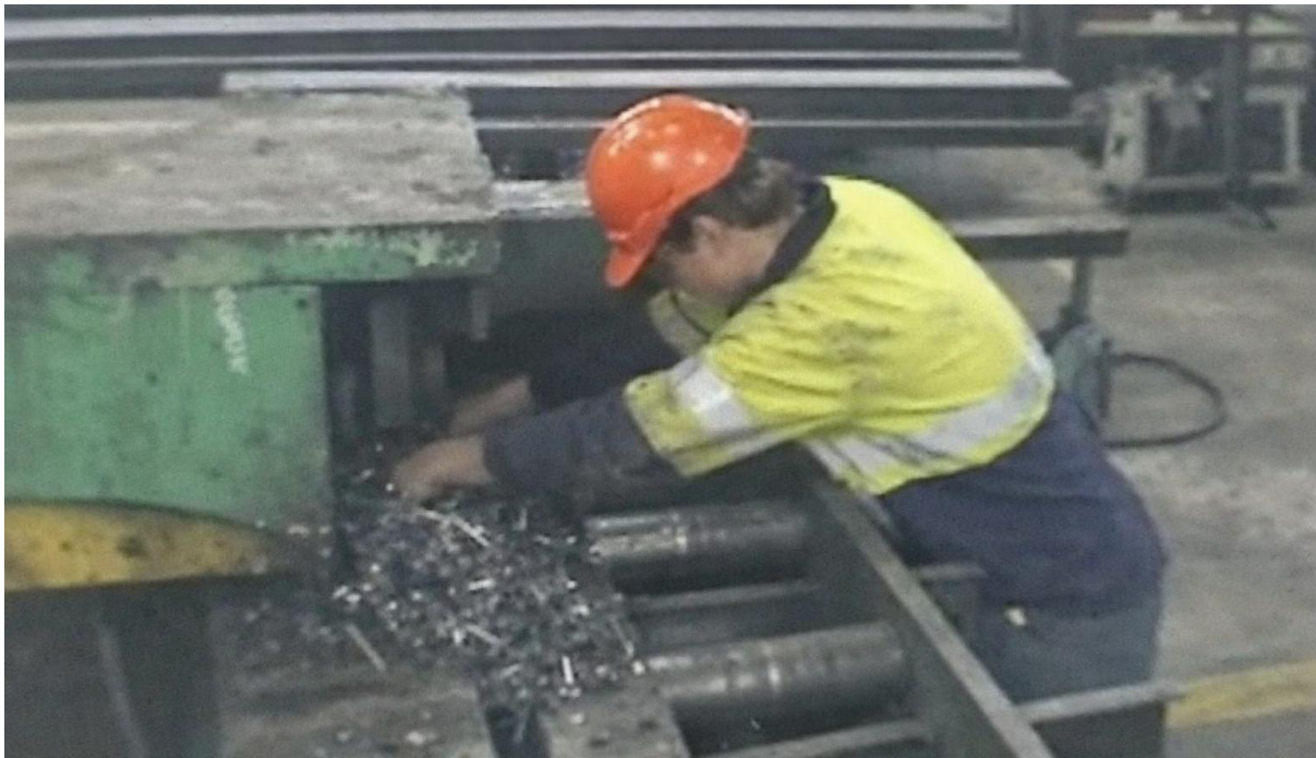
Figure 1. Drill line drop end where the cadet reached in to clear a jammed lintel and swarf without isolating the line. No leading hand was on the floor at the time, the revised isolation procedure had not been inducted, and competency sign-off for unsupervised operation had been deferred twice during the split-site transition. Source: CTV Footage still.
